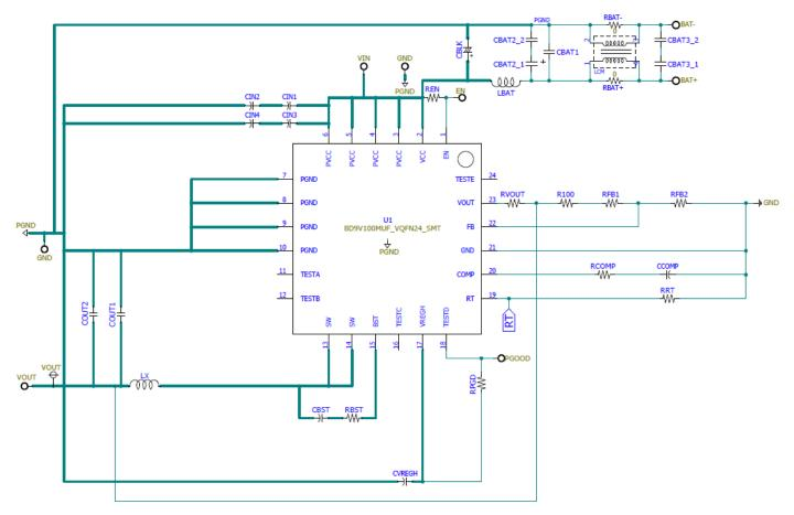
Fig 2: BD9V10xMUF-EVK-001 Evaluation Board Schematic
