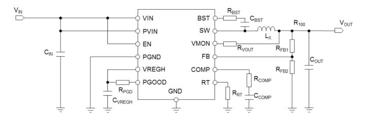
Fig 3: BD9V10xMUF Reference Application Circuit
