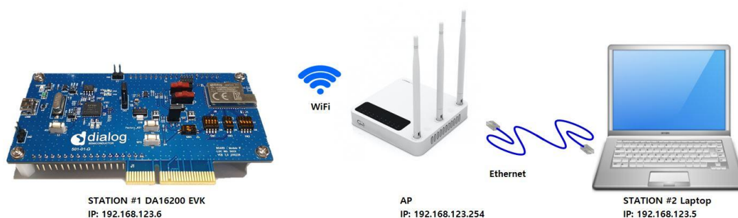
Figure 46: Throughput Test Environment
