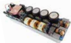
STEVAL-7BIDIRCB 7 kW bidirectional AC-DC converter based on totem pole PFC and CLLC
