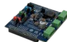
STEVAL-SPSA068 PMIC evaluation board based on SPSA068
