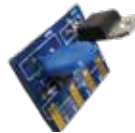
STDES-OVP001 +/- 6 kV Lightning Surge Protection
