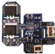
STDES-DIS001V1 Active discharge of high-voltage 400 V bus
