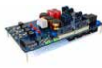
STEVAL-11BID1KCB 11 kW bidirectional battery charger based on three phase two level PFC and DAB converter
