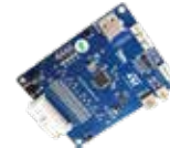
AEK-POW-BMSNOTX Non-isolated Battery Management node
